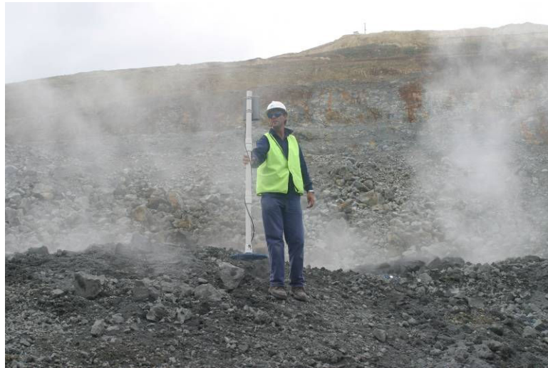
Figure 4 - Locating the transmitters on a freshly blasted muck pile
