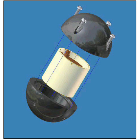
Figure 2 – Expanded view of plastic “transmitter” ball
