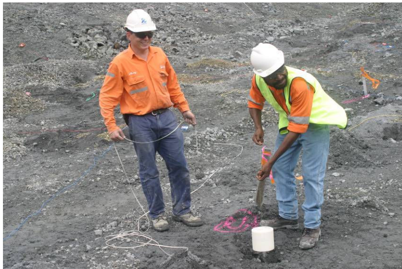
Figure 3 - Installation of blast movement monitor (white cylinder at hole collar)
