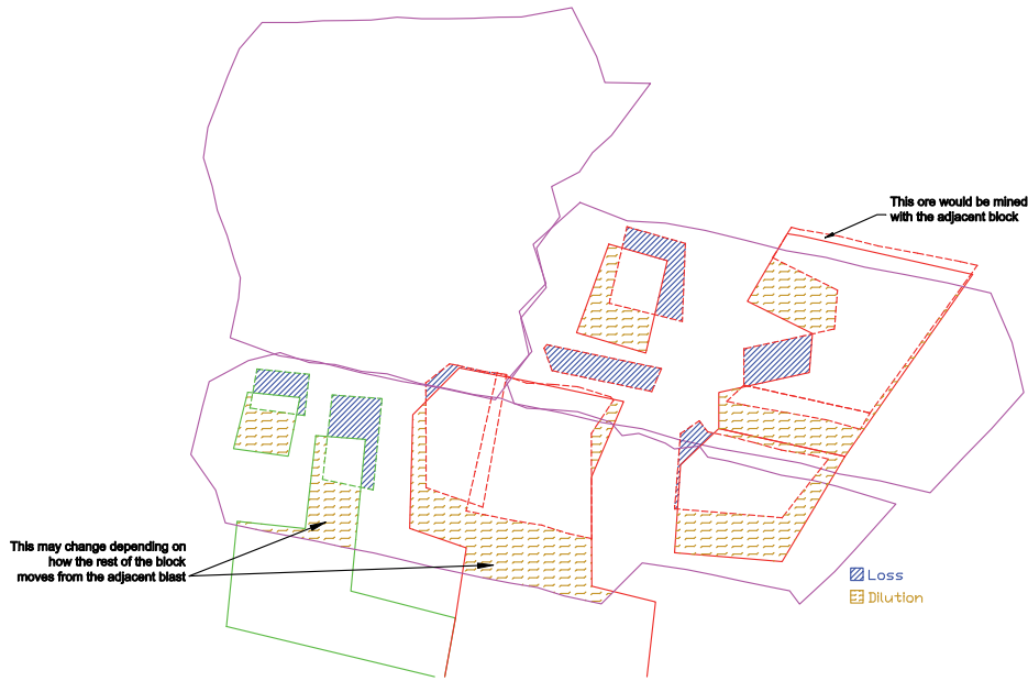
FIG 8 - Loss and dilution for the bottom flitch of all monitored blasts, April 2005.
