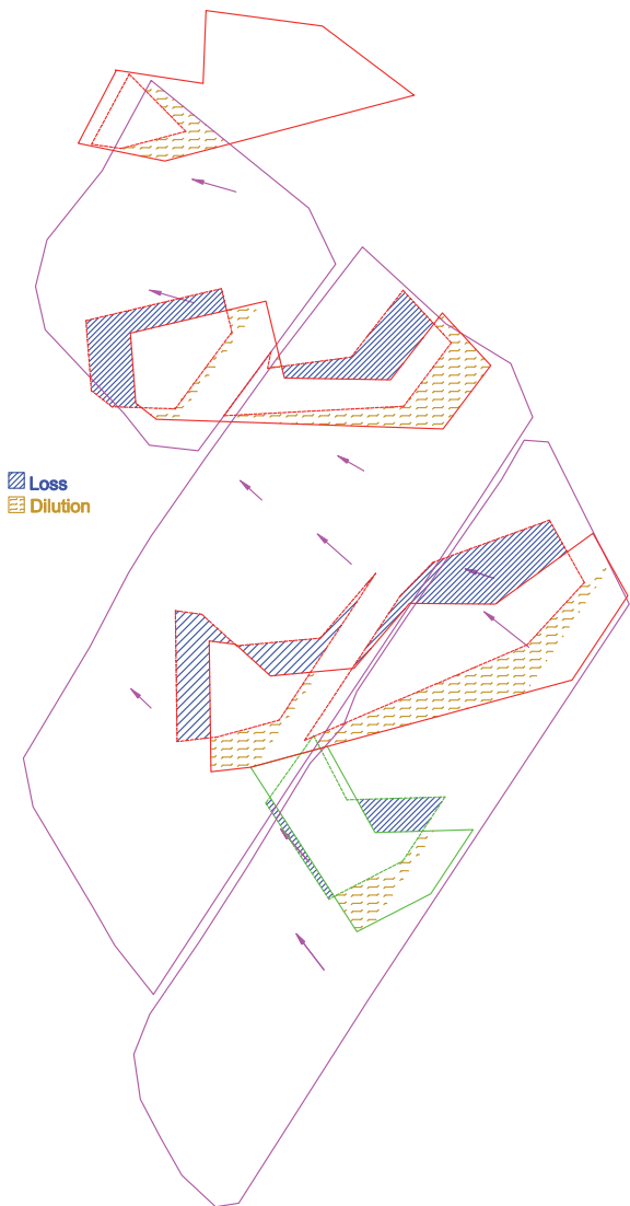
FIG 9 - Diagram showing areas of ore loss and dilution for bottom flitch ore, December 2005.
