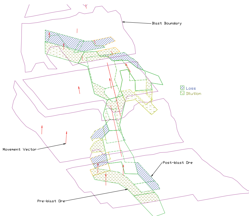
FIG 7 - Loss and dilution for the bottom flitch of blast 260-31, August 2003.
