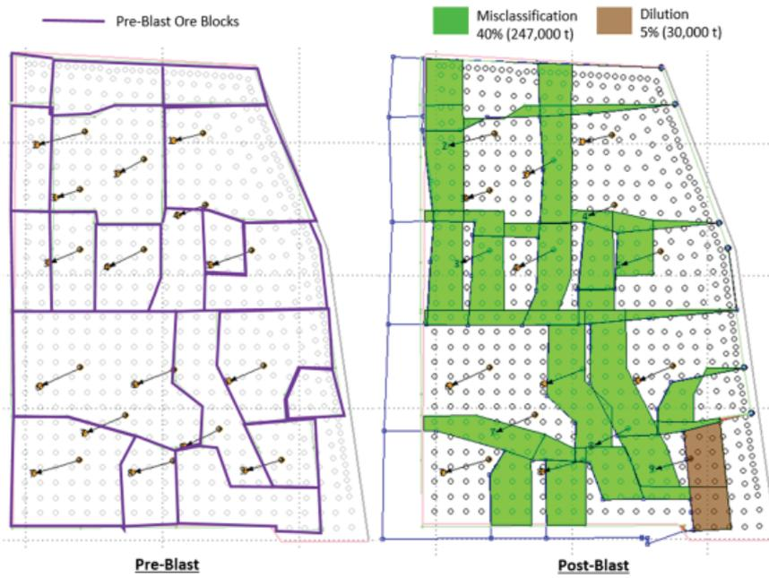
FIG 3 – Mine A Blast ore blocks translated using 16 Blast Movement Monitors placed throughout the pattern.
