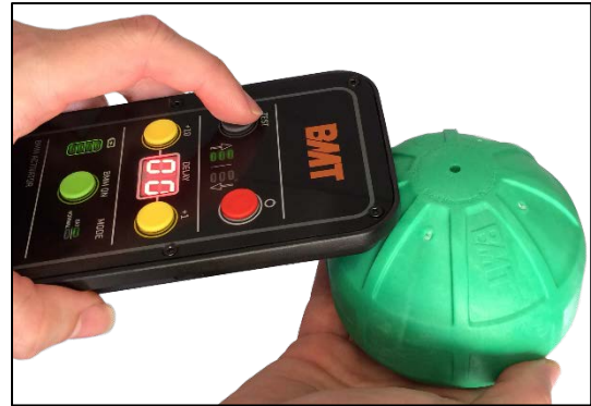
Place the Activator on the BMM; press TEST to check if a BMM works.
